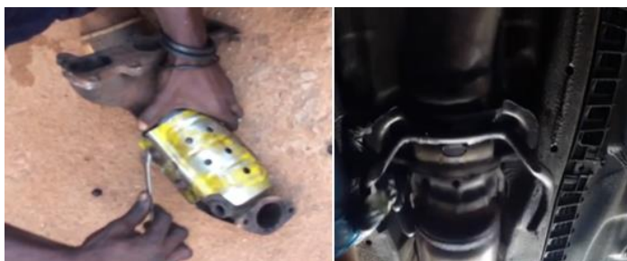
• Fig. 1. Installation of the refurbished Catalytic Converters to Exhaust Systems
