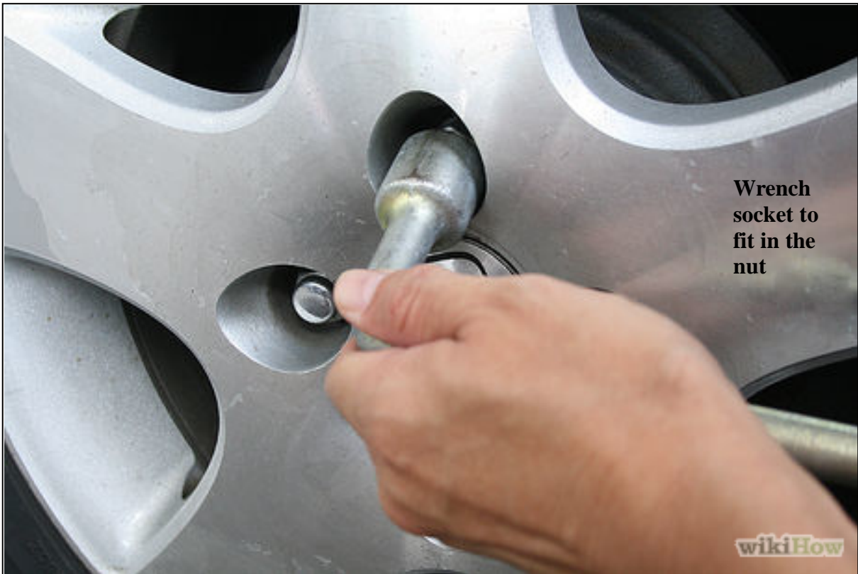
Figure no. 6 Removing nut using T-wrench
