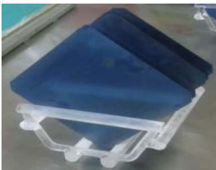
Figure 7: Phosphorous doped on P type Si wafer from diffusion chamber.
