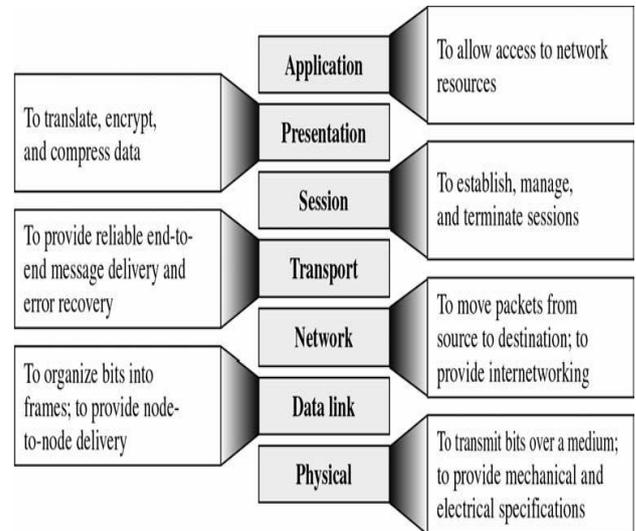
Figure2: Layers of Network model and their functions.
