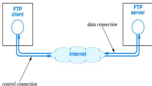
Figure4: FTP Client and server connection.
