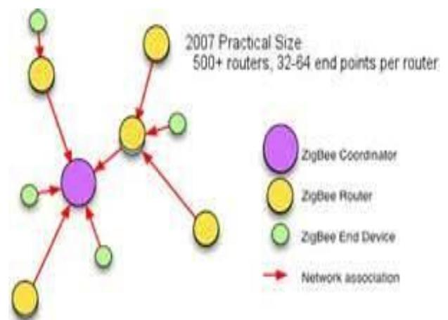
Figure7: Zigbee Network Architecture
