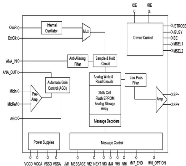
Figure6: APR9600: Block Diagram
