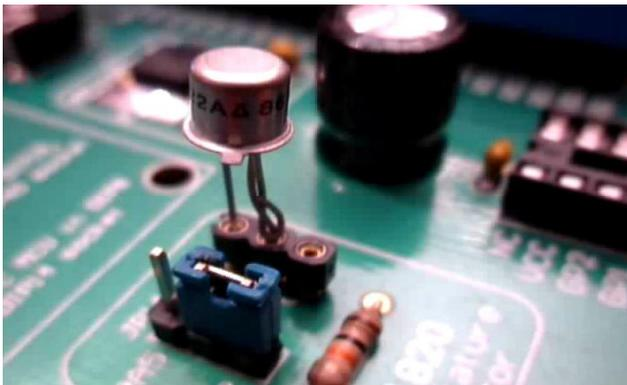
Figure9: Temperature sensor.
