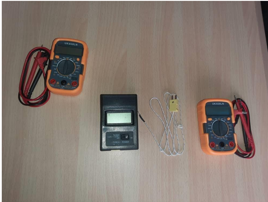
Figure 4: Apparatus used for measuring the performance of our TEG: Left and Right are multi-meters used for currents/voltage measurements, while, the Centre equipment is the digital thermometer for temperature measurement.
