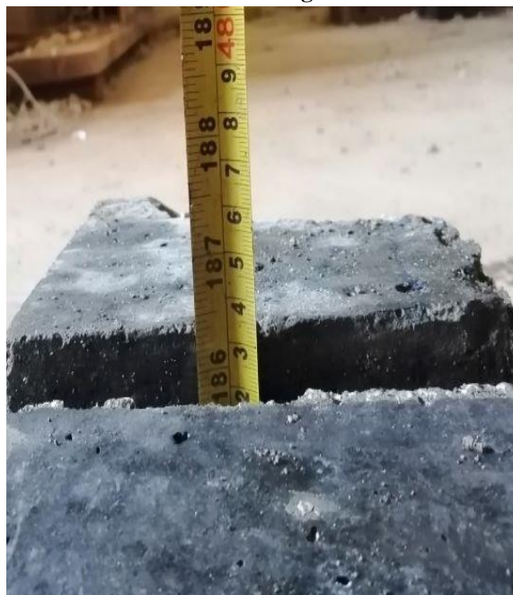
Plate 4: Height difference between control and EPScrete specimen
