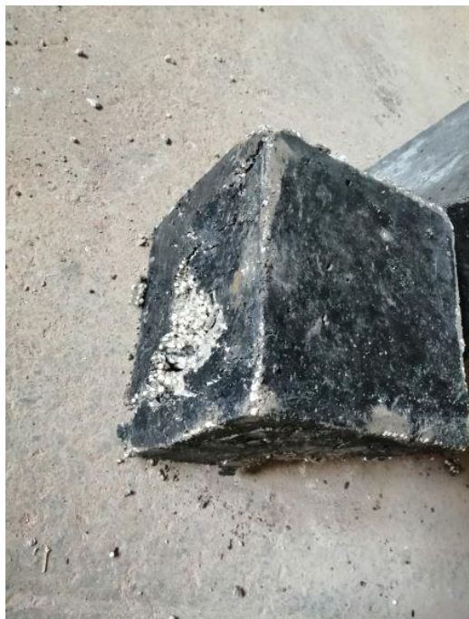
Plate 1: Bulging of EPScrete upon loading
