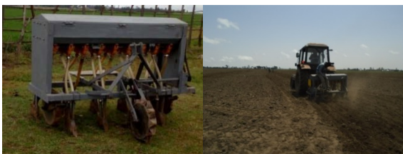
Figure 1. Fabricated tractor mounted row planter
