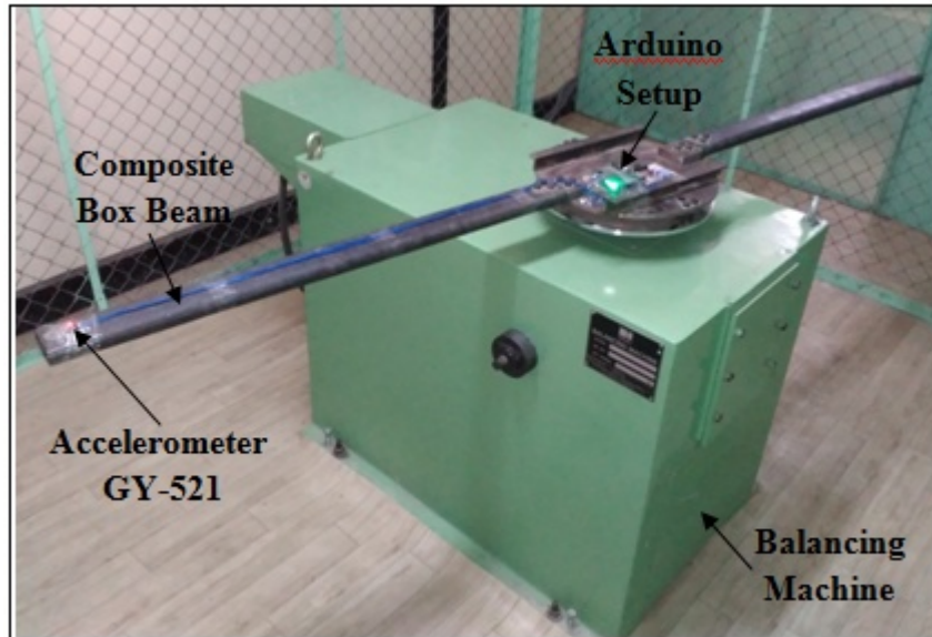
Figure 1 Experimental setup for acceleration measurement using GY-521 Accelerometer
