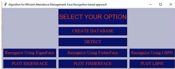
Figure shows the GUI that was made using Tkinter, as an interactive Application, using Python as a programming language and making use of OpenCV
