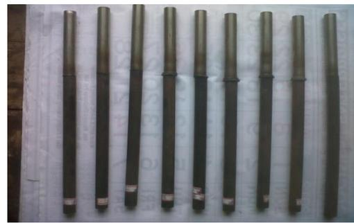
Fig.1: Specimens of joint between SS316 and EN-8 as per L<sub>9</sub>3<sup>3</sup>
