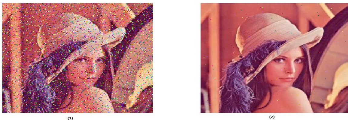
Figure-3: (1) Lena image with 10% impulse noise (2) Filtered image using proposed method
