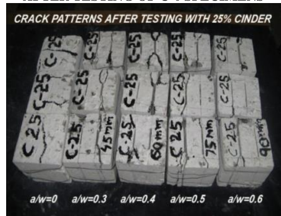
PLATE 11. VIEW SHOWS THE CRACK PATTERNS AFTER TESTING OF C-25 SPECIMENS
