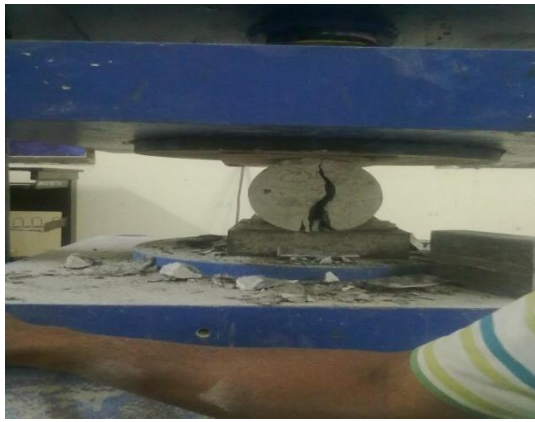
PLATE 7. VIEW SHOWS THE SPLIT TENSILE STRENGTH AFTER TESTING
