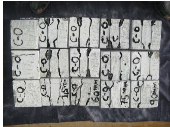
PLATE 10. VIEW SHOWS THE CRACK PATTERNS AFTER TESTING OF C-0 SPECIMENS
