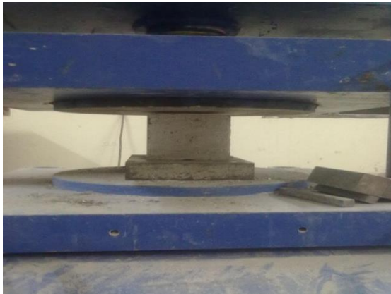
PLATE 2: TEST SETUP FOR CUBE COMPRESSIVE STRENGTH TEST BEFORE TESTING
