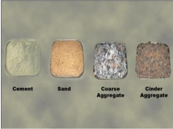
PLATE 1: INGREDIENTS OF CONCRETE
