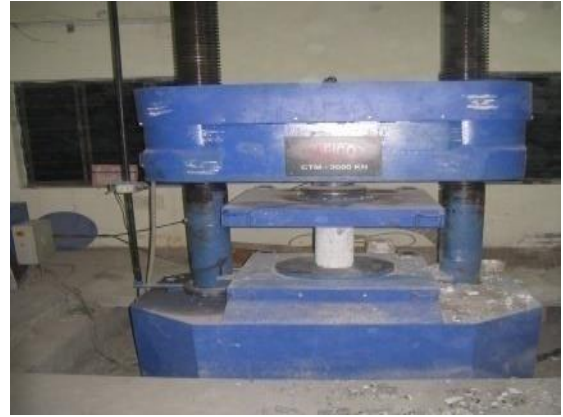
PLATE 4: TEST SET UP FOR CYLINDER COMPRESSIVE STRENGTH BEFORE TESTING
