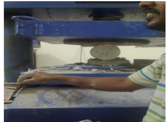
PLATE 6: TEST SET UP FOR CYLINDER SPLIT TENSILE STRENGTH BEFORE TESTING
