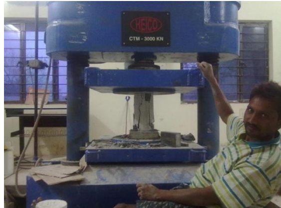
PLATE 5. VIEW SHOWS THE CYLINDER AFTER TESTING
