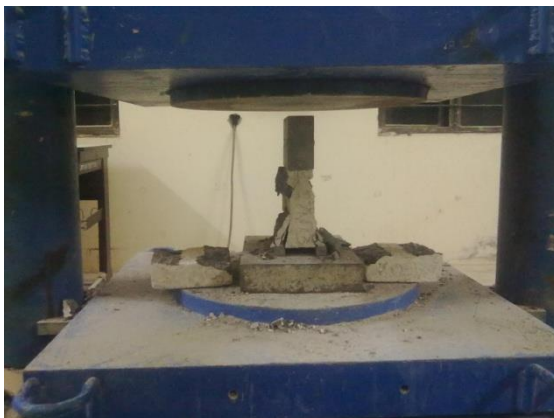
PLATE 9. VIEW SHOWS THE MODE-II FAILURE OF NOTCHED CUBE
