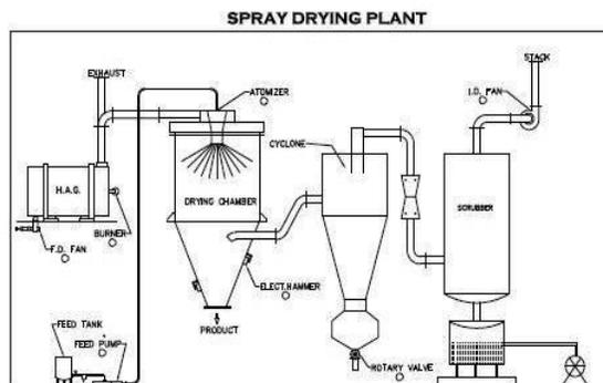
The main components of the drier were the feed system, air compressor with blower, rotary disk atomizer and peristaltic pump. The feed system of drying air constituted of a blower and
