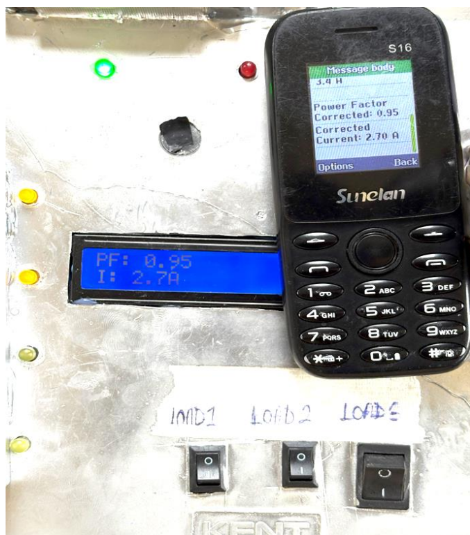
Fig. 15 Implemented system, Load 3 (inductive) after power factor correction
