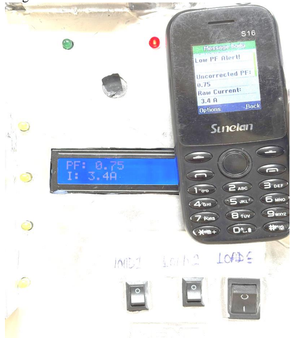
Fig. 14 Implemented system Load 3 (inductive) operating at low power factor before correction
