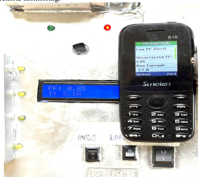
Fig. 11 Implemented System, Load 1 (inductive) at low power factor before correction
