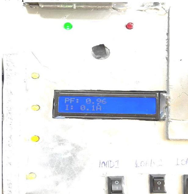
Fig. 13 Implemented system Load 2 (resistive) operating at a good power factor
