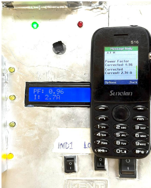
Fig. 12 Implemented system Load 1 (inductive) after power factor correction.
