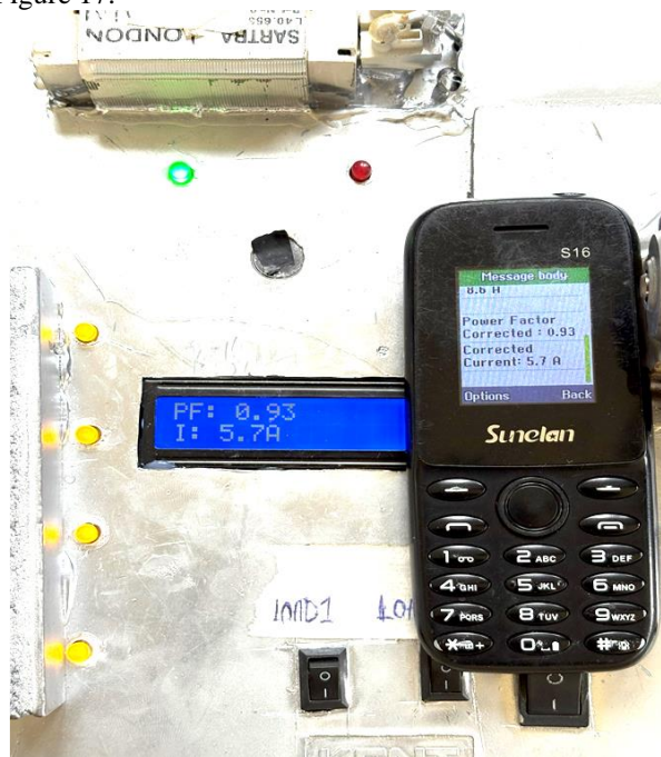
Fig. 17 Implemented system, all Loads (Mixed) after power factor correction
