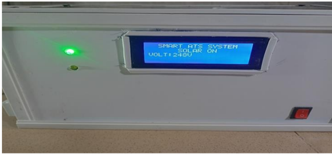
Fig. 9 Experimental test when the Grid is off and the Solar source relay was activated to supply power to the connected load
