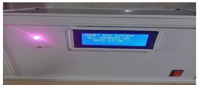
Fig. 8 Experimental test of the system when all sources are available, but on the Grid, relay is activated to supply power to the connected load
