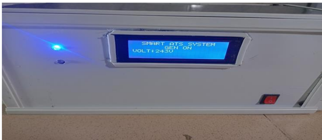
Fig. 10 Experimental test of the system when both Grid and Solar are unavailable and the Generator source relay is activated
