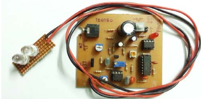
Figure 15. Transmitter Circuit on PCB with the output LEDs.
