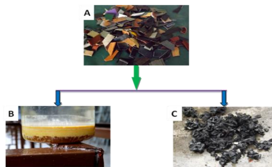
Figure 3.0 Pyrolysis of leather; (A) shredded leather wastes, (B) pyrolytic oil from leather, (C) char
