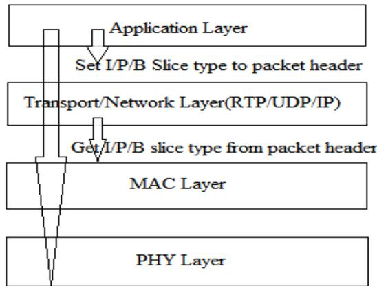
Fig. 1 Cross Layer Architecture [2]
