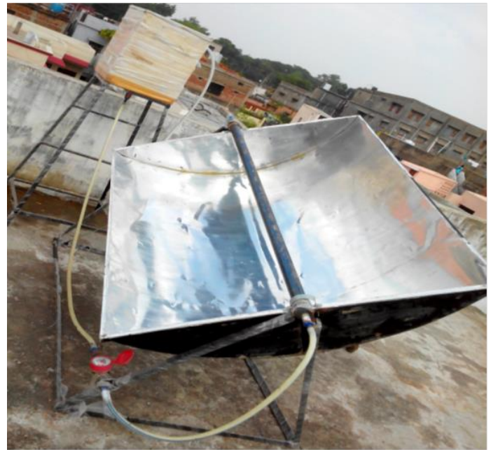
Figure : The parabolic trough system with storage tank
