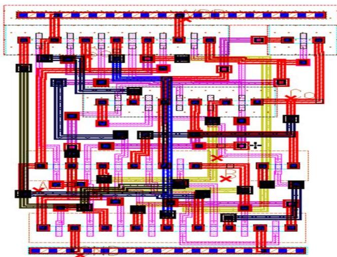
Fig. 7. Layout of the SRCPL full-adder.
