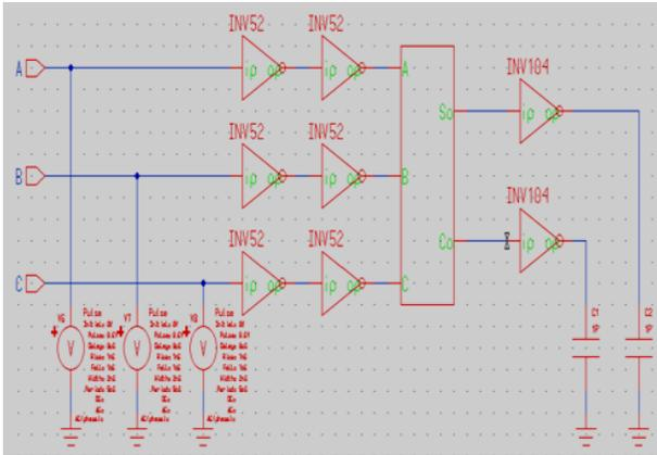
Fig 5. Test bed used for simulating the full-adders under comparison.
