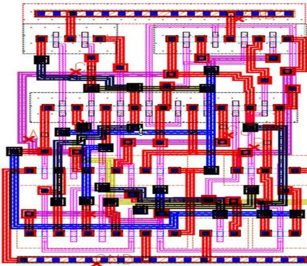
Fig. 6. Layout of the DPL full-adder.
