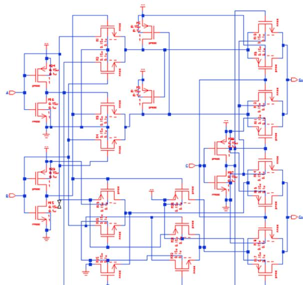
Fig. 4. Full-adder designed with the SR-CPL logic style.
