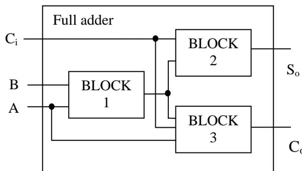
Fig.1. Full-adder cell formed by three main logical blocks.
