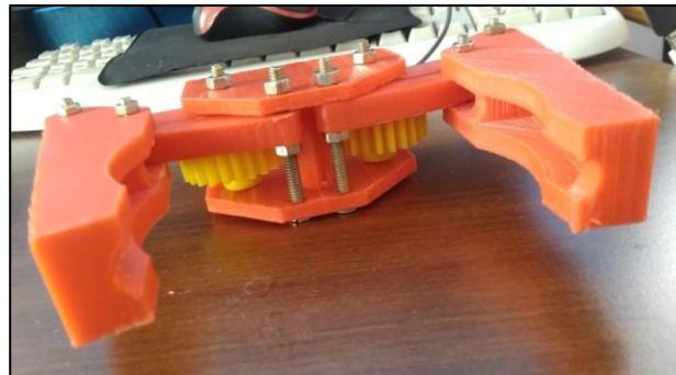
Fig 3.32 Motor with helical gear which drives spur gears
