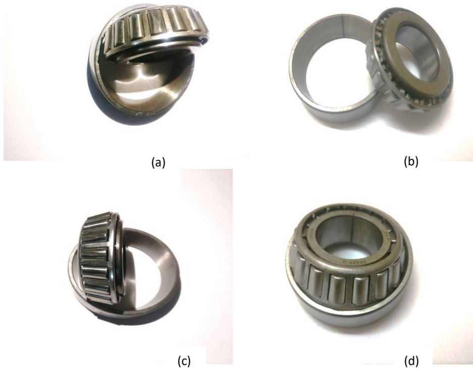
Figure 3. Different defects (a) Single roller defect (b) Outer race EDM cut (c) Double roller defect(d) Inner race EDM cut
