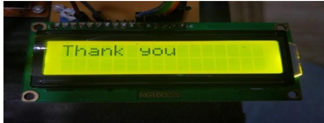
Fig.4.6 Acknowledgement message displayed on the LCD screen for the courier driver
