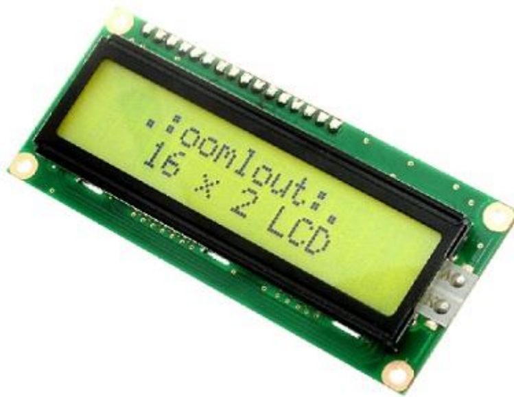
Fig 3.8 LCD 16x2 character display
