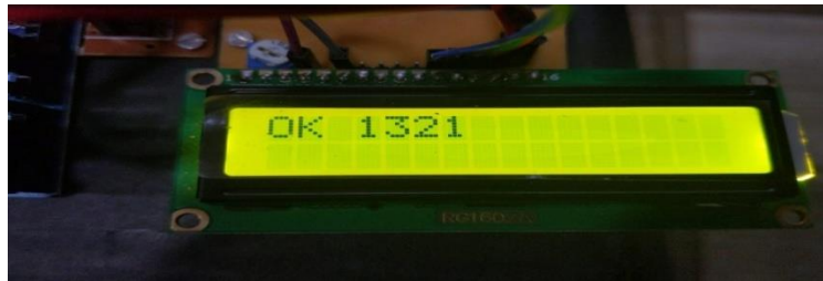
Fig.4.4 OTP displayed on the LCD screen
