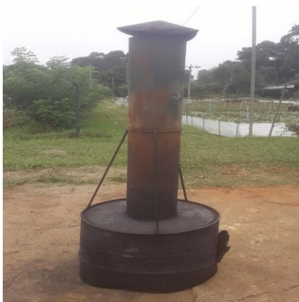
Plate 3-3 Instrument to prepare partially Burn Rice Husk
