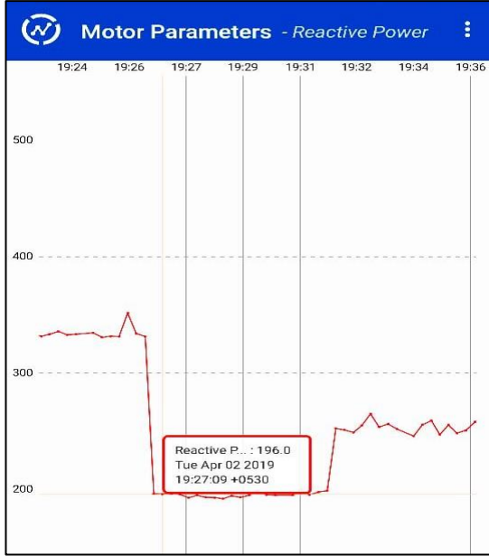
Fig. 4.6 Reactive Power Reading for Load 1
