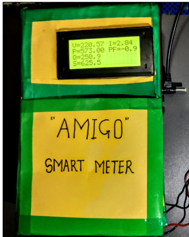
Fig. 3.17 Hardware Model of SMART METER
