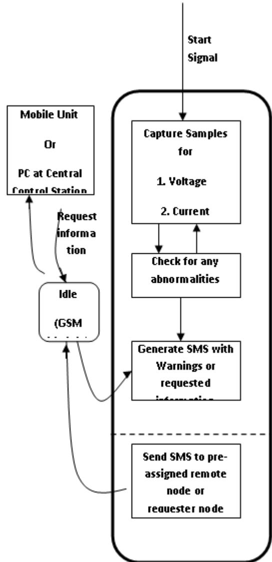
Fig. 4 State Chart diagram of DHU algorithm
