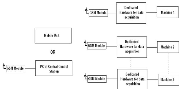
Fig. 1 Block diagram of PC based wireless monitoring of multi-machine system
