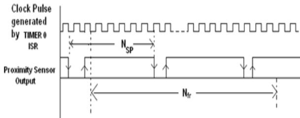
Fig. 3 Timing diagram to measure speed
