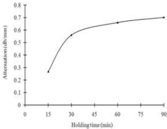
Figure 4: Dependence of attenuation coefficient of DSS on holding time at 1300°C
