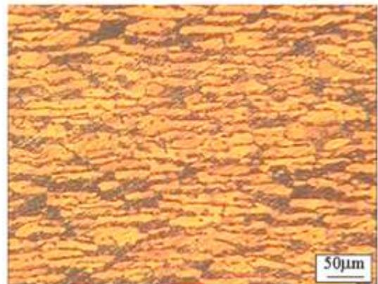
Figure 2: Optical micrograph of duplex stainless steel in as-received condition. Dark etched regions are ferrite and white regions are austenite.
