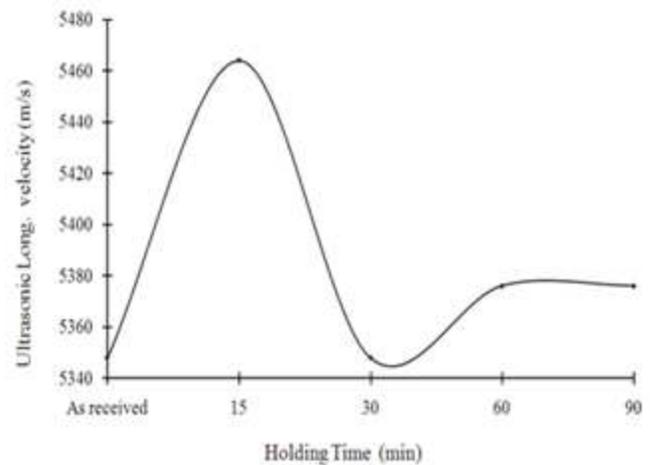
Figure 6: Variation in longitudinal wave velocity in DSS with holding time at 1300°C
