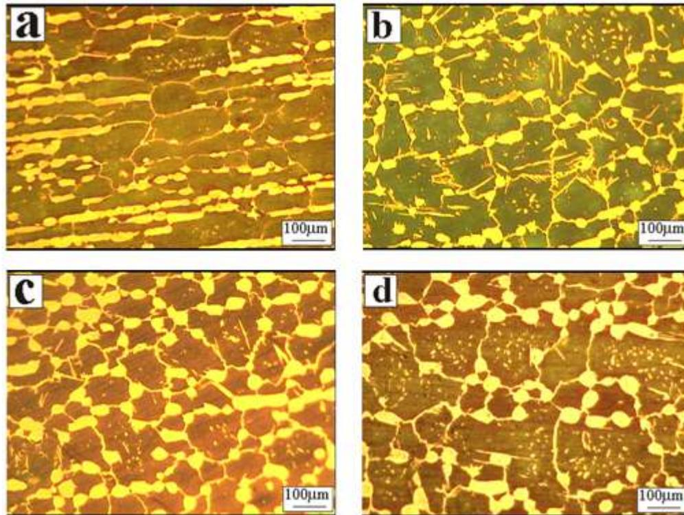
Figure 3: Microstructure of duplex stainless steel held at 1300°C for different duration, (a) 15min (b) 30min (c) 60min (d) 90min and water quenched
