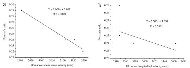
Figure 10: Correlation between (a) Poisson's ratio and ultrasonic shear wave velocity (b) Poisson's ratio and ultrasonic longitudinal wave velocity, in DSS
