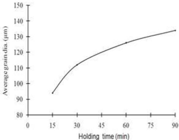
Figure 5: Effect of holding time at 1300°C on average grain size of DSS
