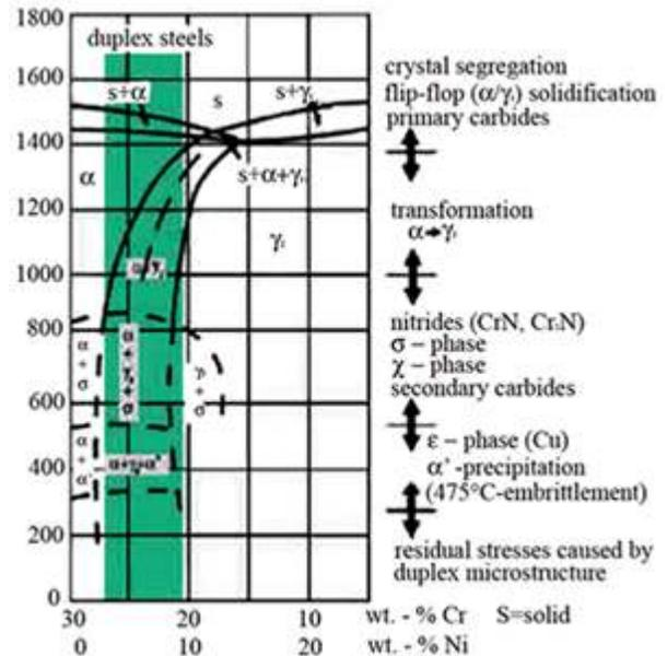
Figure 1: Pseudo binary diagram of duplex stainless steel for 70% Fe-Cr-Ni [19]
