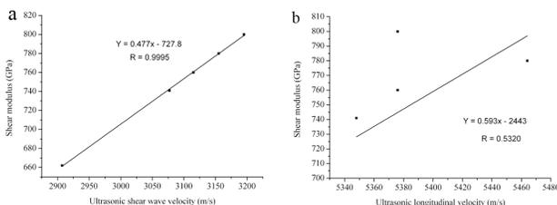
Figure 8: Correlation between (a) shear modulus and ultrasonic shear wave velocity (b) shear modulus and ultrasonic longitudinal wave velocity, in DSS
