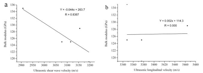
Figure 9: Correlation between (a) Young's modulus and ultrasonic shear wave velocity (b) Young's modulus and ultrasonic longitudinal wave velocity, in DSS
