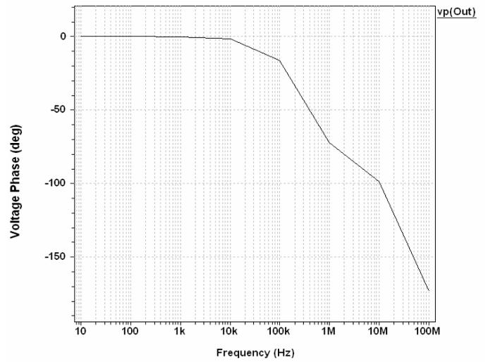
Fig 3 Voltage Phase of Bulk Driven Balanced OTA
