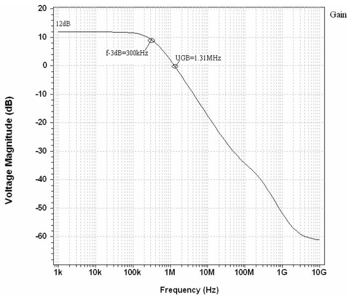
Fig 2 Voltage Gain of Bulk Driven Balanced OTA
