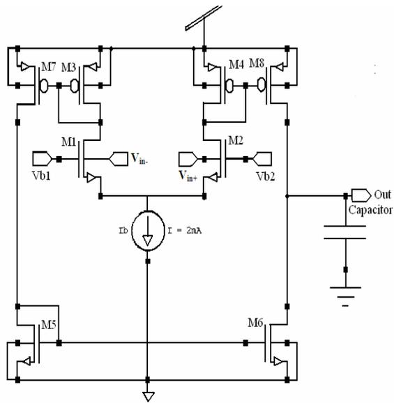
Fig 1 Bulk Driven Balanced OTA
