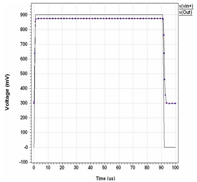
Fig 4 Slew rate of Bulk Driven Balanced OTA
