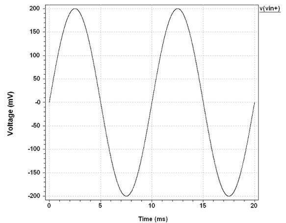
Fig 5(a) Input Voltage Swing of Bulk Driven Balanced OTA
