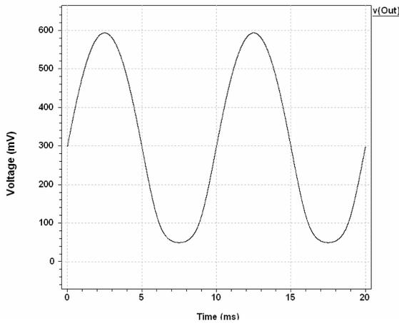
Fig 5(b) Output Voltage Swing of Bulk Driven Balanced OTA
