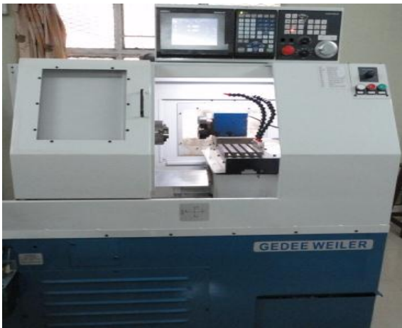
Figure 2.: CNC turning center. (MITSUBISHI-EZ Motion NC E60)
