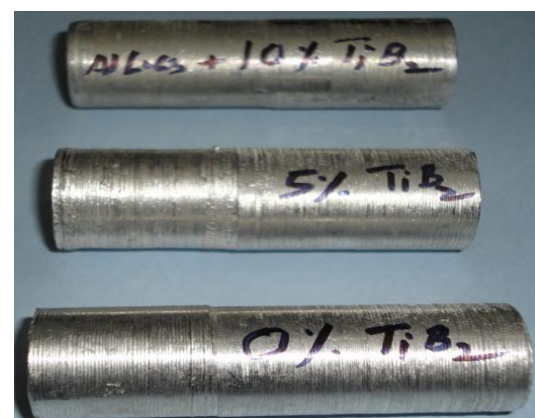
Figure 1: Composite Material 0, 5 & 10 wt% TiB_2 Reinforced with Al6063.
