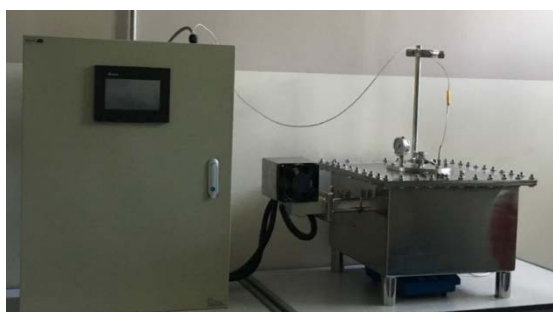
Figure 5. Exterior of the microwave reactor with its power control panel
