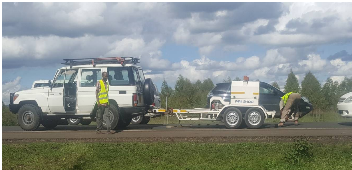
Plate 1: Pavement Surface Deflection Measurement Using FWD Equipment
