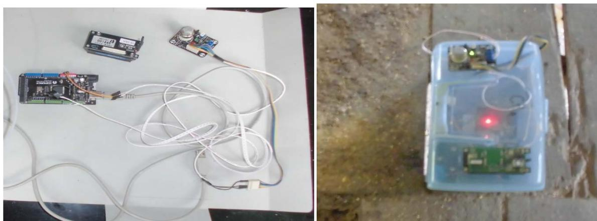
Figure 1. NH3 sensor, temperature, humidity and Speed Direction (Teguh, R. 2016)
