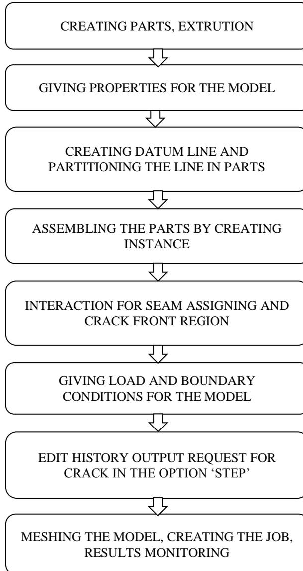
**Fig 1: Flow of work in Abaqus**
