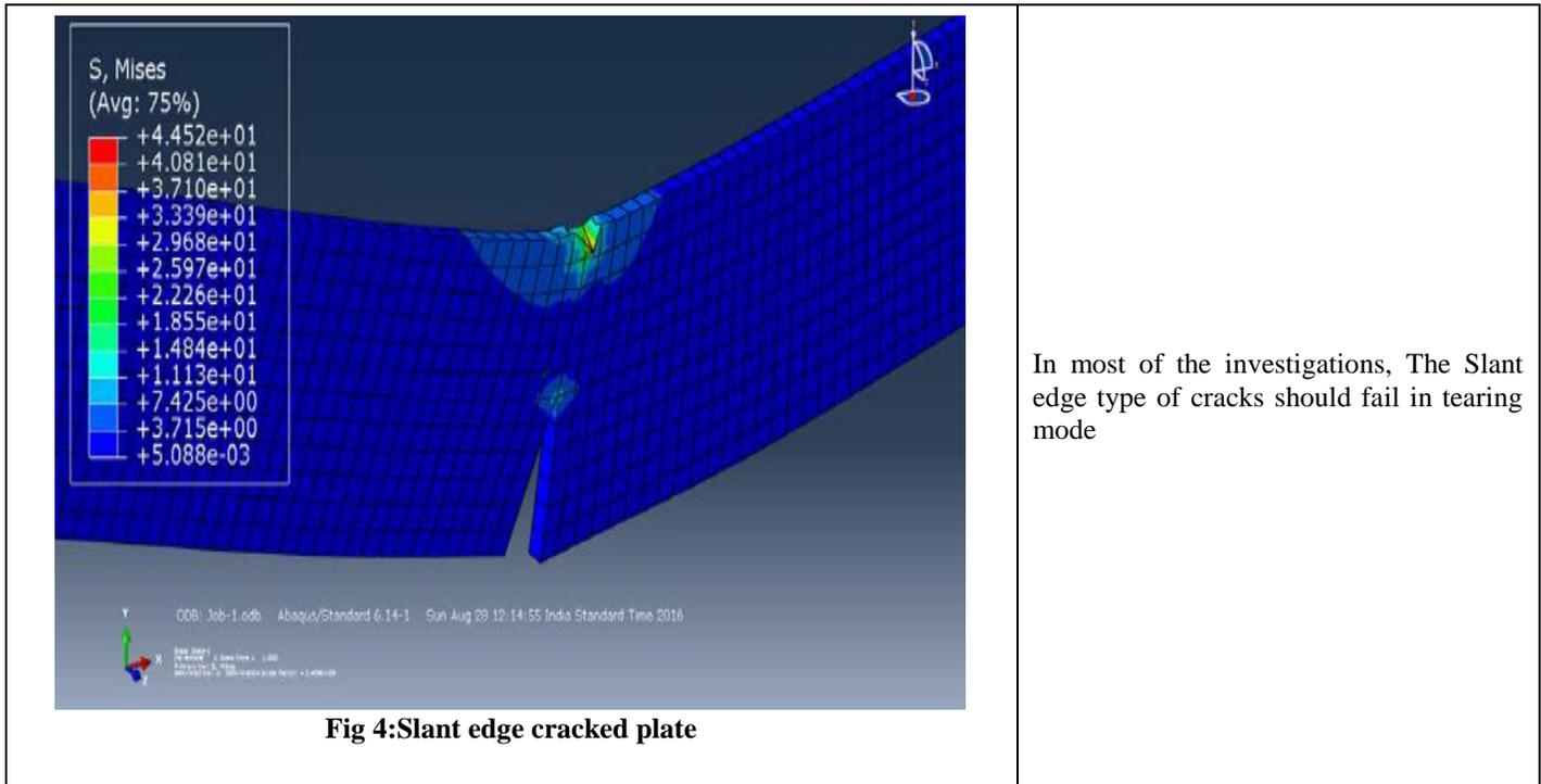
**Fig 4: Slant edge cracked plate**
