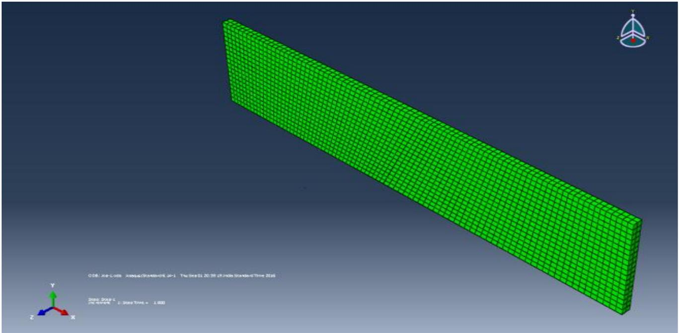
**Fig 3: Meshing of plate**
