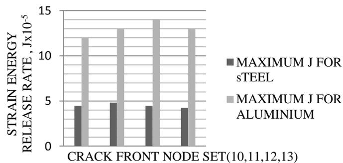
**Fig 2: Comparison of max J value for both the materials**
