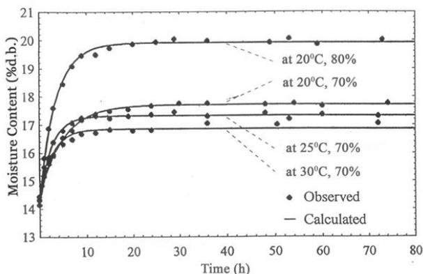
Figure 3: Water adsorption characteristics of polished rice under fluidizing conditions
