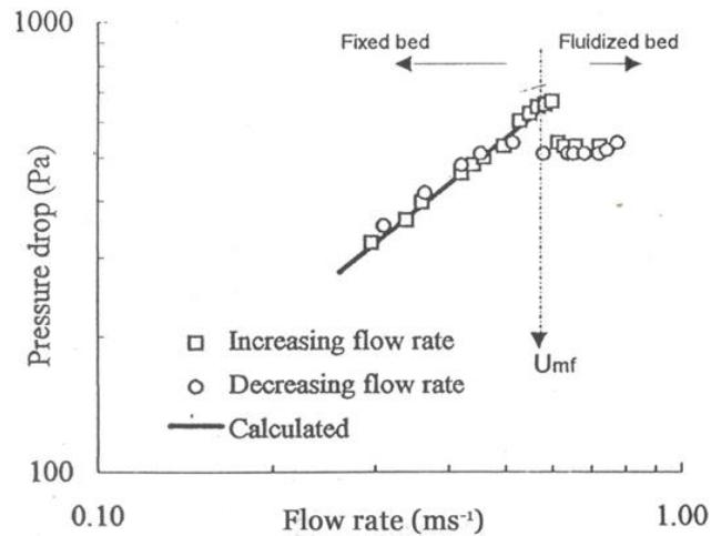
Figure 2: Pressure drop versus flow rate of polished rice fluidized in air
