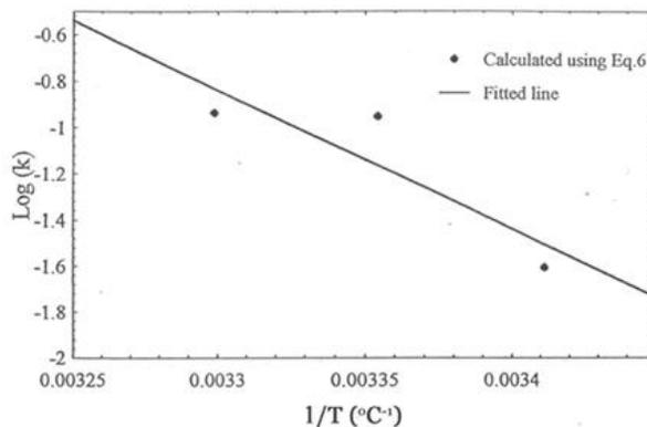
Figure 4: Arrhenius plot of sorption coefficient ( $k$ ) at 70% relative humidity
