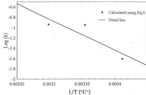
Figure 4: Arrhenius plot of sorption coefficient ( $k$ ) at 70% relative humidity
