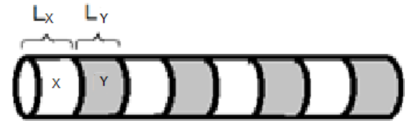
Fig. 1. The superlattice structured nanowire in which X=SrTiO 3 and Y= anatase TiO 2
