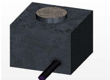
Fig. 3 Mesh Model of Plenum Chamber
