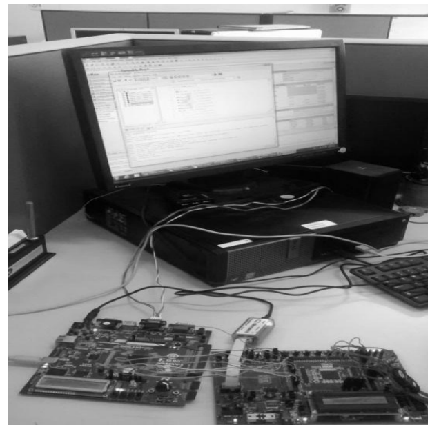
Figure 5: Xilinx board(Master), ACTEL board (Slave) connected by LVDS lines
