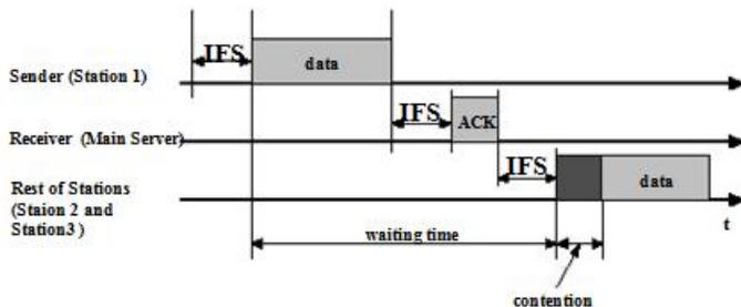
Figure 3 backoff Timer (BOT) and Inter Frame Space (IFS) Mechanism
