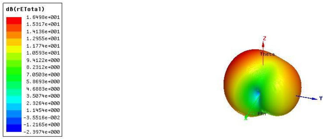
Gain of the antenna at various phases at its operating frequency 1.6GHz
