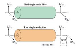
These two local polarization modes travel at different velocities causing a pulse spreading in digital systems. The so induced DGDs vary randomly along the fiber and in time, leading to a statistical behavior of PMD, both in time and wavelength. At a given time, the DGD values vary randomly with wavelength. The PMD value is the average of the DGD values. While the individual values can shift from one time to another the overall distribution, hence the average is assumed to be fixed.
