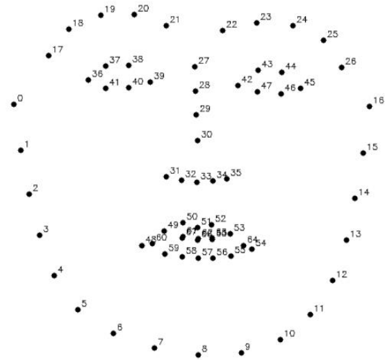
Figure 1 Eye detection by the landmarks 36, 39, 42 and 45 of the shape predictor provided by Dlib
