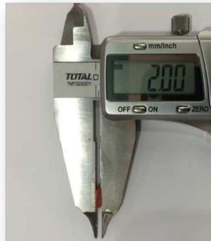
Figure (2) digital vernier measure the block dimension
