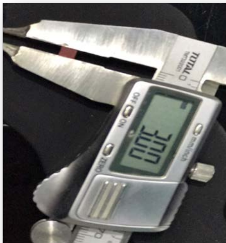
Figure (2) digital vernier measure the block dimension
