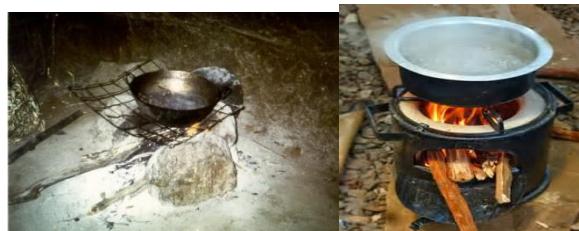
Figure 2:Three stones firewood stove Figure 3:Portable firewood Conservation stove. Source: Researcher Source: Researcher
