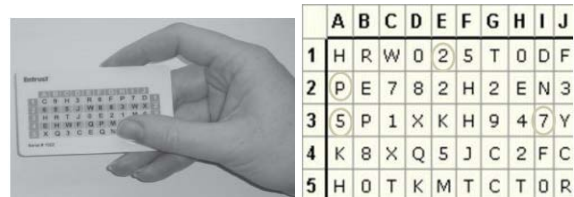
FIGURE 2. SAMPLE ENTRUST IDENTITYGUARD GRID AUTHENTICATION SCHEME (A) SAMPLE PRINTED ENTRUST CARD AND (B) SAMPLE ENTRUST GENERATED GRID CARD
