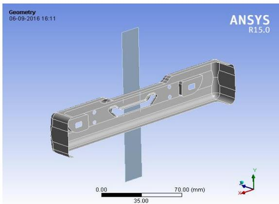
**Fig. 3 Geometry of the BUMPER**
