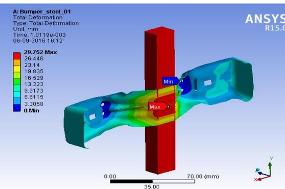
**Fig. 6 Deformation of the BUMPER**
