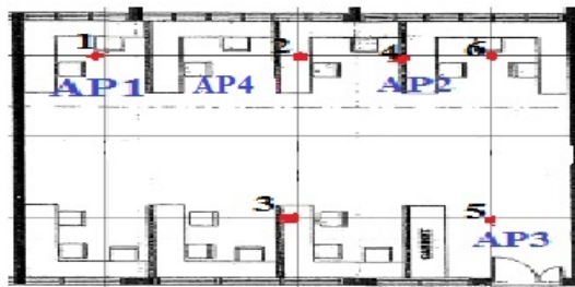
Figure 1: Location of four APs and the measurement points in the Computer laboratory room
