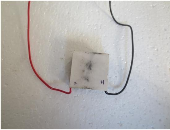
**Fig2: A typical thermopile**
