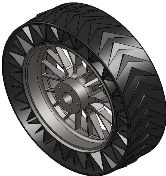
Fig1. Isometric view of the wheel design. The design procedure is performed on the SolidWorks design package based on the calculated parameters.
