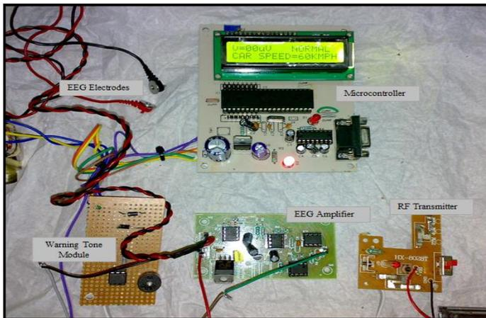
**Figure 5: Hardware Setup**
