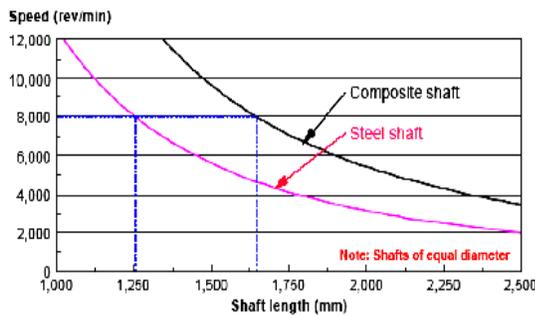
**Fig.3. The effect of shaft length on critical speed**
