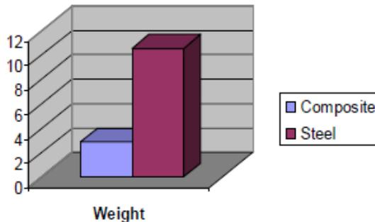
**Fig.4. Mass comparison between steel and composite shaft**
